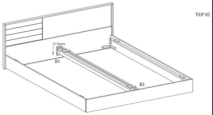
Place the Part -D in between U-batten at postion B1 and B2 respectively as shown in fig.
