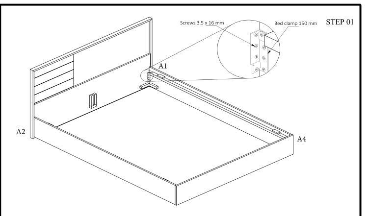
Fix the Part -A, Part-Cand Part -F with bed clamp of 150mm using screws of 16mm with the help of screw driver at position A1,A2,A3 and A4 as shown in Fig.
