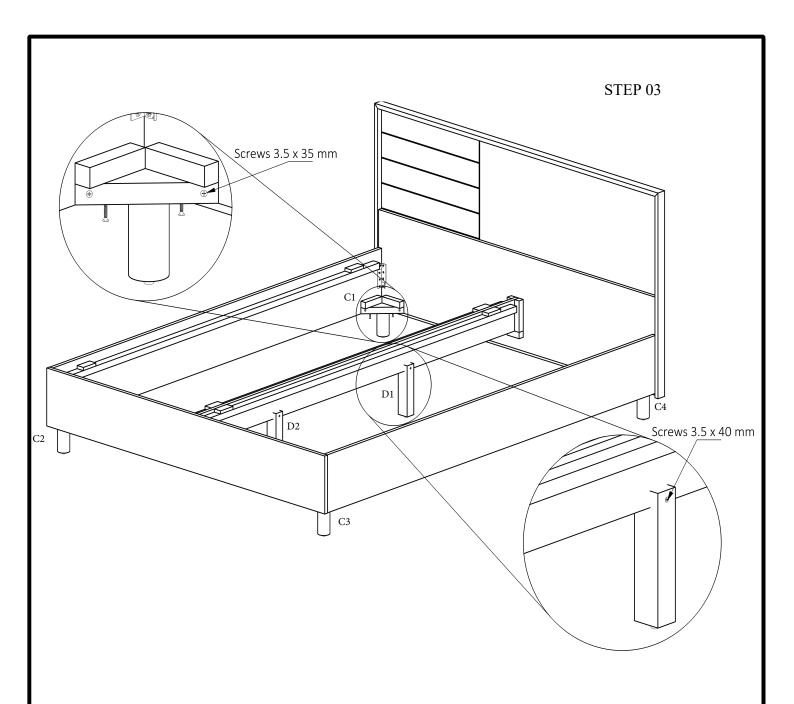
Fix the Part -B(Leg) using screw of 35 mm at position C1,C2,C3&C4.Also fix Part -E at position D1 & D2 using screw of 40mm with the help of screw driver at position D1 and D2 diagonally as shown in Fig.
